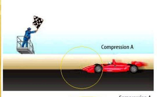
The Doppler effect occurs when the source of a sound wave is moving relative to a listener.
