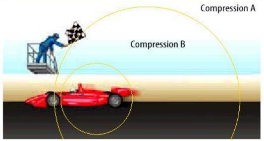
B The car is closer to the flagger when it creates compression B. Compressions A and B are closer together in front of the car, so the flagger hears a higher-pitched sound.
